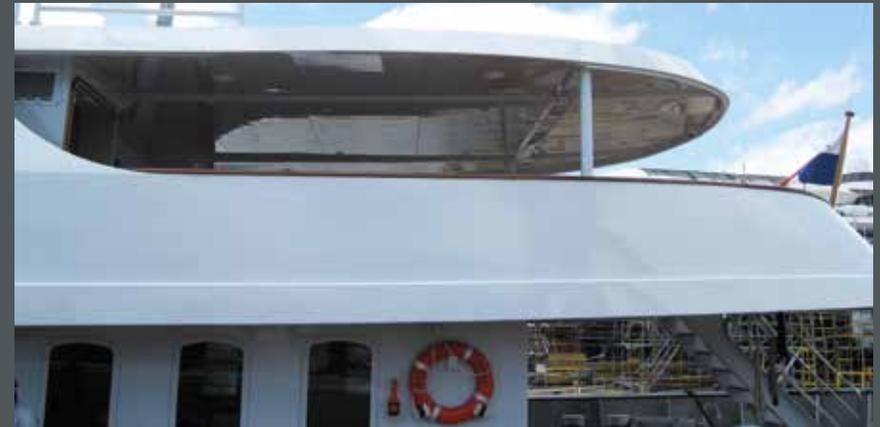
**CONSTRUCTION PROCESS** Helicopter deck extension with an aluminium structure and installation of new zero speed stabilizers.
